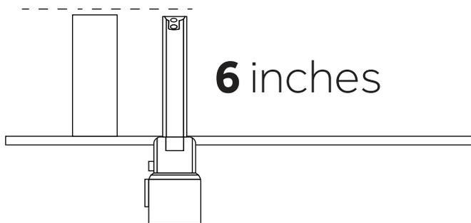
3. When the floor is finished, measure and cut the drain pipe to the appropriate length for the type of drain that is being used.
