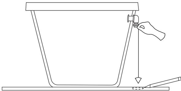
2. Move the tub away from the installation location so that the plumbing can be installed. Place the drain pipe at the appropriate height for waste and overflow piping. To determine this, you will need to temporarily fit your drain pipe into the tub and measure from the floor to the center of the drain pipe.
