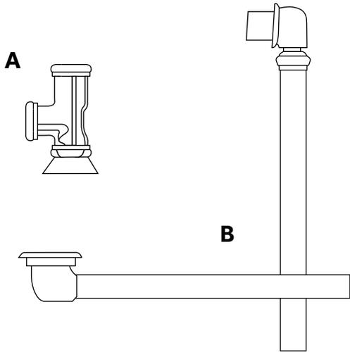
7. Measure and mark each pipe so that the end of the pipe reaches at least a little bit over halfway into the overflow tee.
