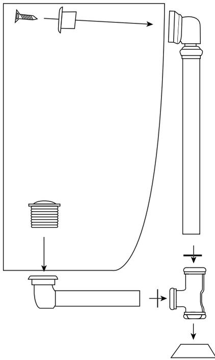
14. When your tub is in place and all the connections have been made, fill the tub with water to check for any leaks from the connections. Verify that the drain and overflow is working properly.
