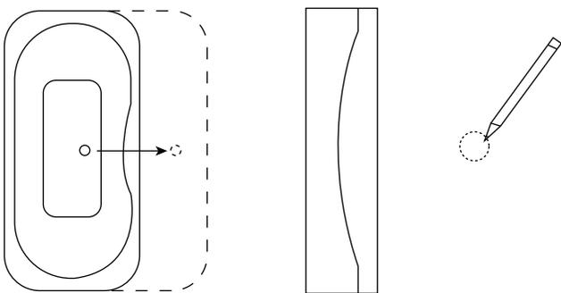
2. Move the tub away from the installation location so that plumbing can be installed. The drain pipe should extend approximately 6" above the finished floor.
