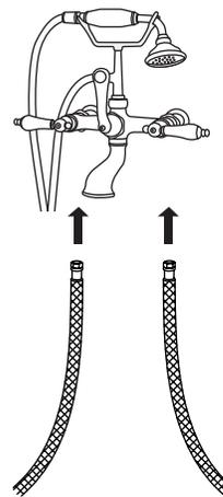
4. Once installation is complete, turn the faucet on for approximately 60 seconds to check for any leaks, and to ensure that hot and cold water are running appropriately. Divert water flow to the hand shower for testing as well.
