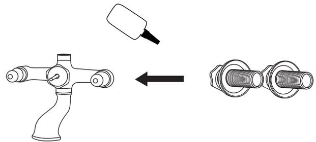
2C. Insert the faucet into its prepared mounting holes. From behind, thread the lock nuts onto the threaded shanks to secure the faucet to the tub.
