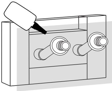
3D. Apply plumber's tape or thread sealant to the threaded outlets on the back of the faucet body. Attach the faucet body to the installed wall mount couplers. Tighten the lock nut firmly using an adjustable wrench.
