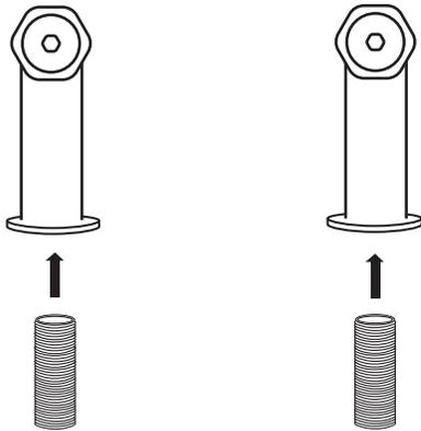
2A. Insert each of the deck couplers into their prepared mounting holes. From underneath, slide the metal washer onto each threaded shank, followed by the lock nut. Thread the lock nut onto the shank until hand-tight. Do not fully tighten yet.
