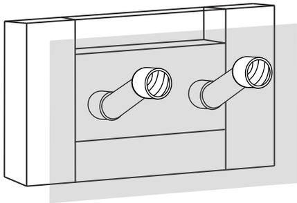
2D. Apply plumber's tape or thread sealant to the exposed threads of the pipe nipples installed in the wall. Attach the provided wall mount couplers to the pipe nipple. Tighten firmly using an adjustable wrench.
